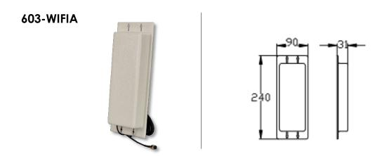
Range boosting antenna which can be added to transmitter at gate and also optionally to the handsfree monitor type. One antenna can boost range by 30%. Comes with 2 metre antenna cable (RG174 with SMA male connector).
